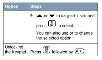
After the keypad is locked, the display shows Keypad Locked and returns to the Home screen.
