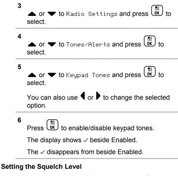
You can adjust your radio's squelch level to filter out unwanted calls with low signal strength or channels that have a higher than normal background noise. Normal is the default. Tight filters out (unwanted) calls and/or background noise; however, calls from remote locations may also be filtered out.
