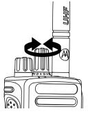
Once the required zone is displayed (if you have multiple zones in your radio), turn the programmed Channel Selector Knob to select the call type.
