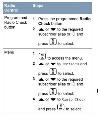
The display shows the Target Alias, indicating the request is in progress. The LED lights up solid green.
