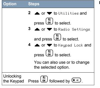
After the keypad is locked, the display shows Keypad Locked and returns to the Home screen.
