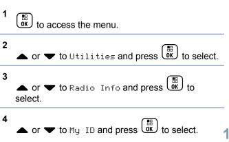
The first line of the display shows the radio alias. The second line of the display shows the radio ID.
