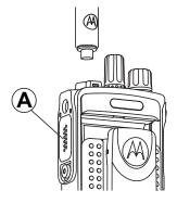
Insert the hooked end of the cover into the slots above the universal connector. Press downward on the cover to seat the lower tab properly into the RF connector.
